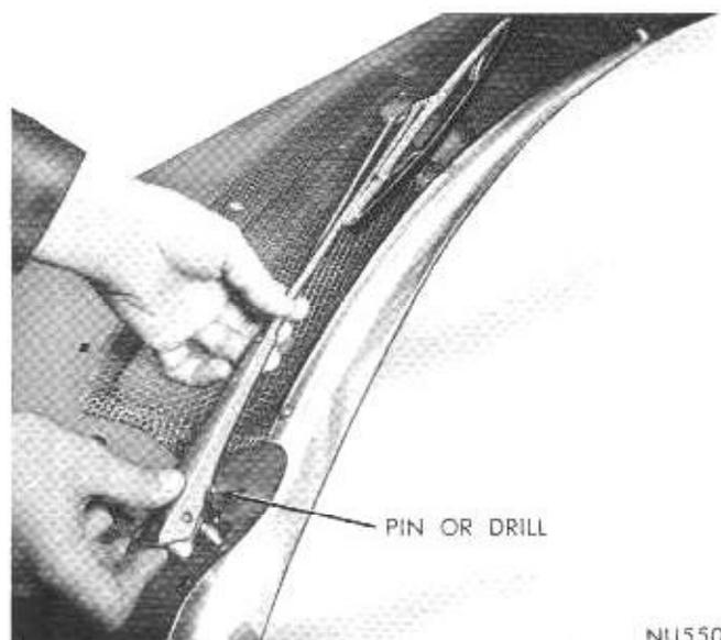
Fig. 1—Removing Wiper Arm and Blade Assembly (Fury)
