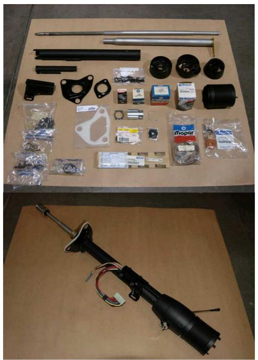
Ignition switch - 3747092 Bearing steering column upper - 2265656 Bearing retainer - 2925491 Key buzzer switch - 2947488 Turn signal lever - 2947953 Cylinder and key package (including door locks) - 3695555 Shaft coupling rebuild kit - 4443436 Can't find the part number for the turn signal switch - it is a 70 only part#.
