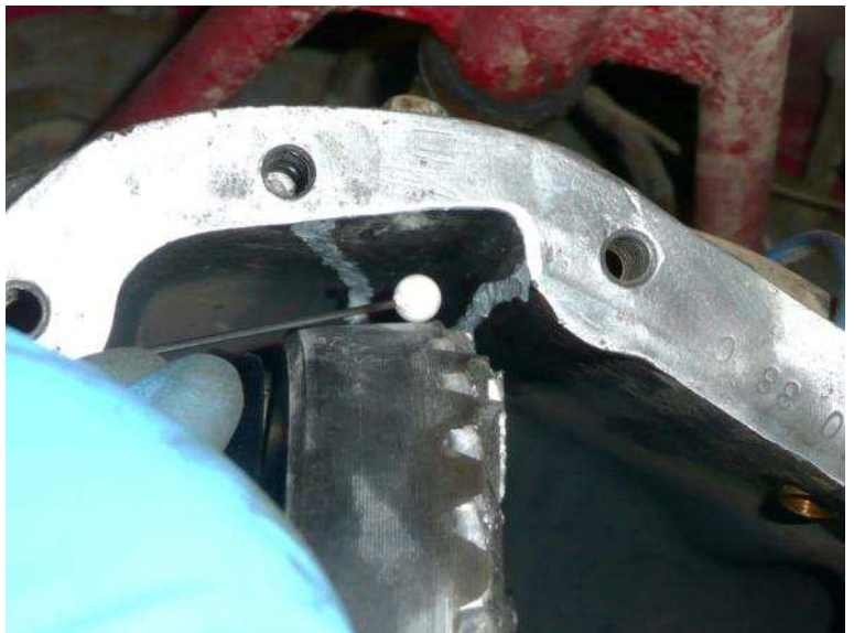
1 MARKING AREAS TO GRIND
