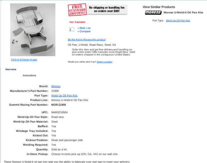
needs. They feature internal baffling that will provide a continuous oil supply to the pickup area. The kits also include a fitting for an oil temperature sending unit. Welding and fabrication are required to assemble the oil pan.
