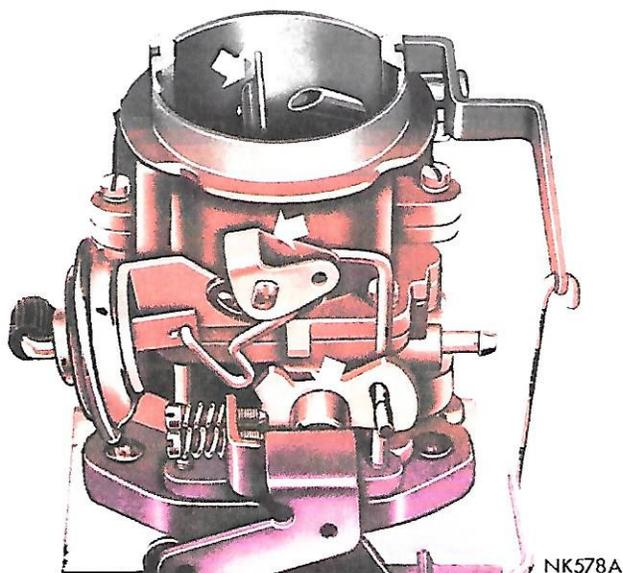
Fig. 44 Choke Valve Shaft and Fast Idle Cam.
