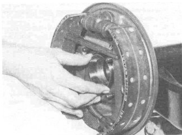
Figure 94 1019-94 Assemble bearing cup into bearing bore of the tube. Make sure the cup backface is against the bearing seat of the tube.
