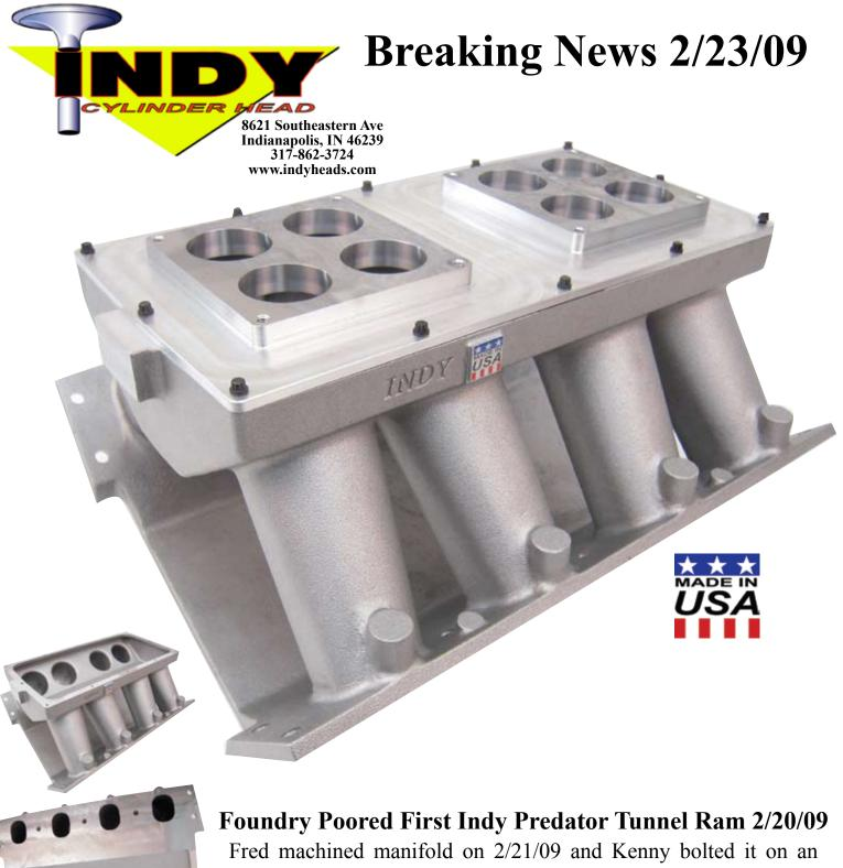
Fred machined manifold on 2/21/09 and Kenny bolted it on an engine 2/23/09. The manifold weights 29 lbs. less top. Top will be billet 6061 T6 Aluminum with 1/2" Aluminum plenum spacers. Bosses for EFI or mechanical nozzles. This week we will finish the cast aluminum valve covers with 1/2" more clearance.
