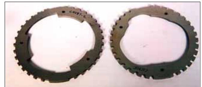
The crank sensor for the 5.7L (right) is considerably different than the one used on the 4.7L (left) and all the other Chrysler engines.
