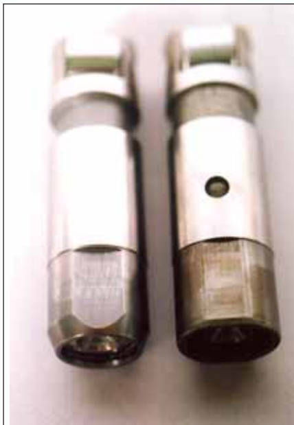
The MDS lifter (right) is unique. It's bigger on top (.7665" vs. .7265" across the flats) and has an extra oil hole in the body.
