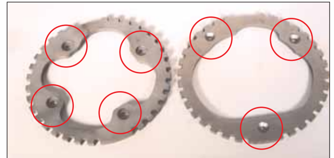
The crank sensor wheel for the 6.1L (left) has four holes instead of the three found on the crank for the 5.7L.
