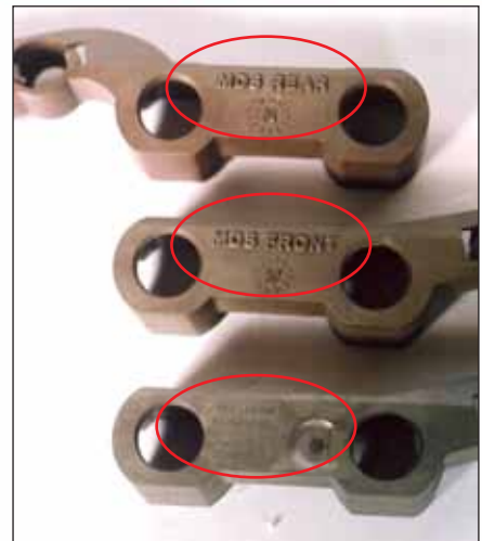
The roller lifters are located with four plastic yokes. There are three different yokes, one for engines without MDS, one for "MDS front" and one for "MDS rear" They are easily identified by the markings found on them.
