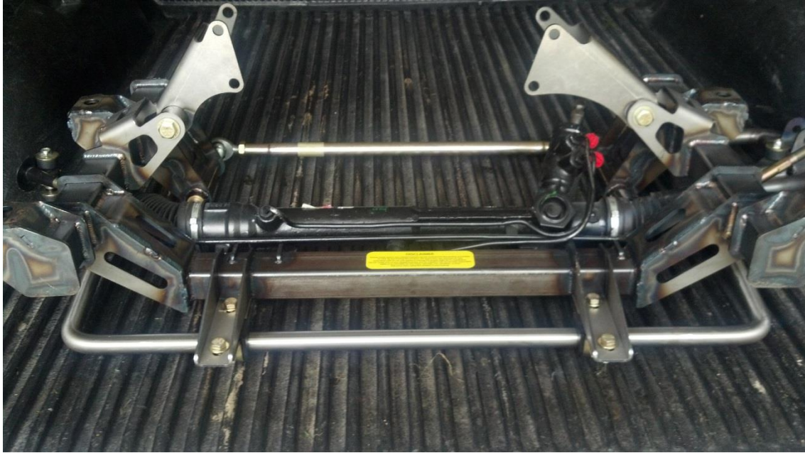
Picture of the new HDK with Schumaker 383/440 spool mount, optional sway bar, and power steering. The production mounts and sway bar come powder-coated gloss black.
