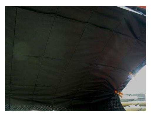
11. Now work down the sides, pulling it gradually from each side, clamping it along the way. As the headliner is pulled outboard, the listing pockets will need to be re-trimmed; trim so that approx. 3/4" of bow is exposed up to the roof side crossmember. Be consistent with this dimension so that the point where the side-to-side stitch seams curves is the same down the whole side. Continue pulling & clamping around the perimeter until the headliner is taught.
