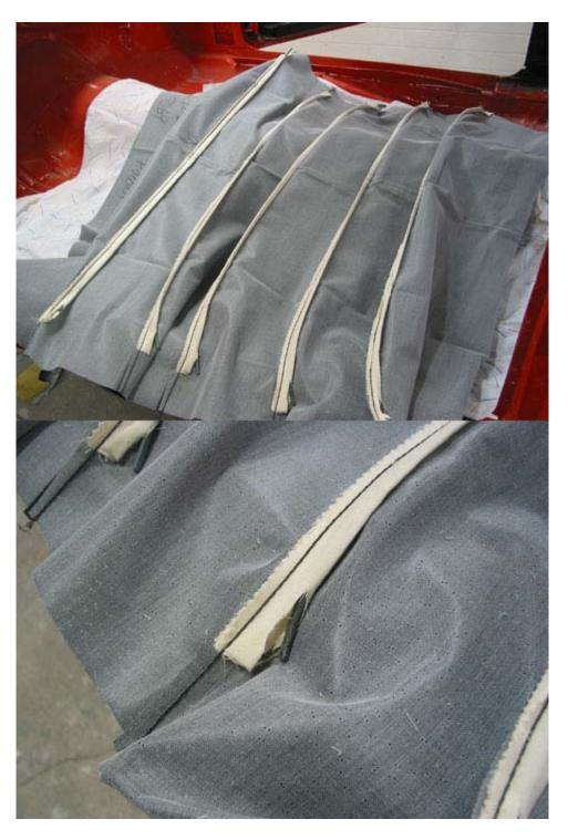
6. Now move the headliner with bows into the car. Place the rear-most bow into the hanger clips. On the rear bow there are 2 small wires with hooks on the ends. One end hooks on the bow and the other presses into a small hole in the rear-most roof crossmember. There's one wire retainer used per side. I like to hook them slightly inboard so that as the headliner is stretched to the sides it will pull them straight.
