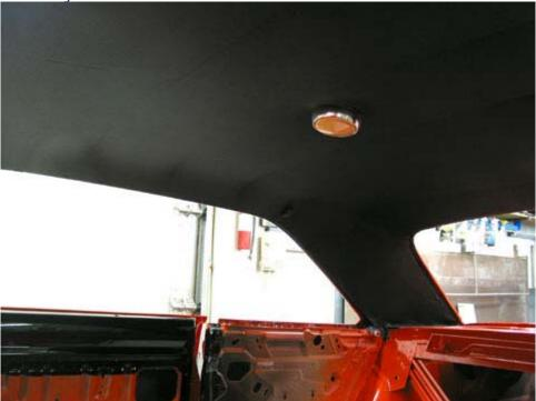
20. Visors, mirror, etc. can be located by feeling through the material to find the indents for the screws. A small needle can also be used to check if you're unsure. Take your time! I haven't scrapped one yet, but I've come close!
